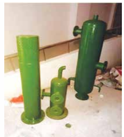
Flash vessel & De-aerator
